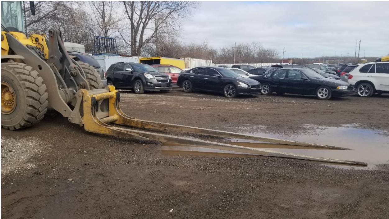
A forklift at Doty has elongated forks to reach under vehicles lengthwise. Source: OIG photo.
