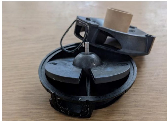
The inside of a disc meter of the kind used in small residential homes. Source: OIG photo.
